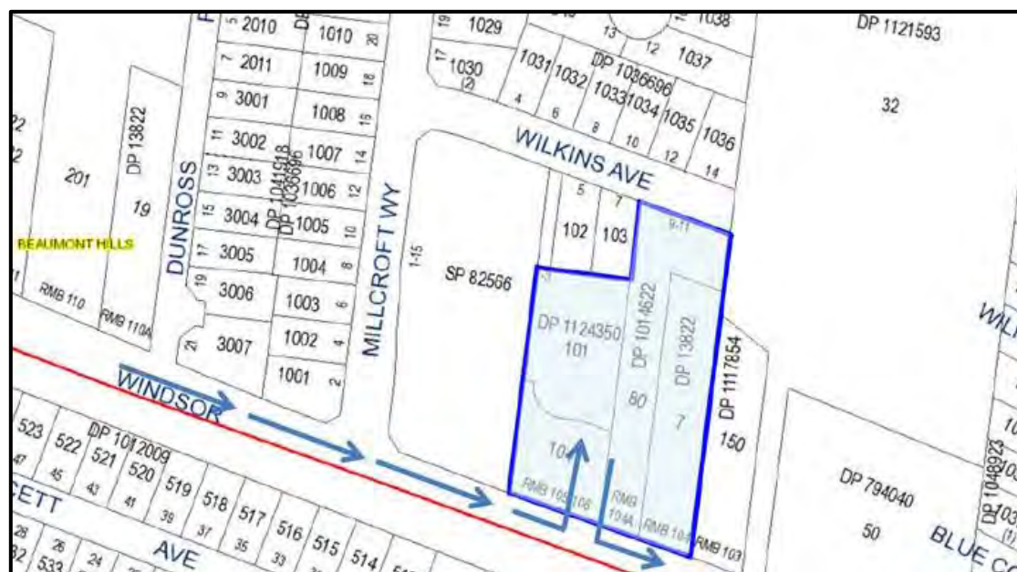
Figure 3 Indicating left in/left out access
